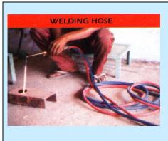
REALON WELDING HOSE meets all requirements for Welding, Brazing and Cutting operations including Oxygen and Acetylene Welding by hand and machine.
